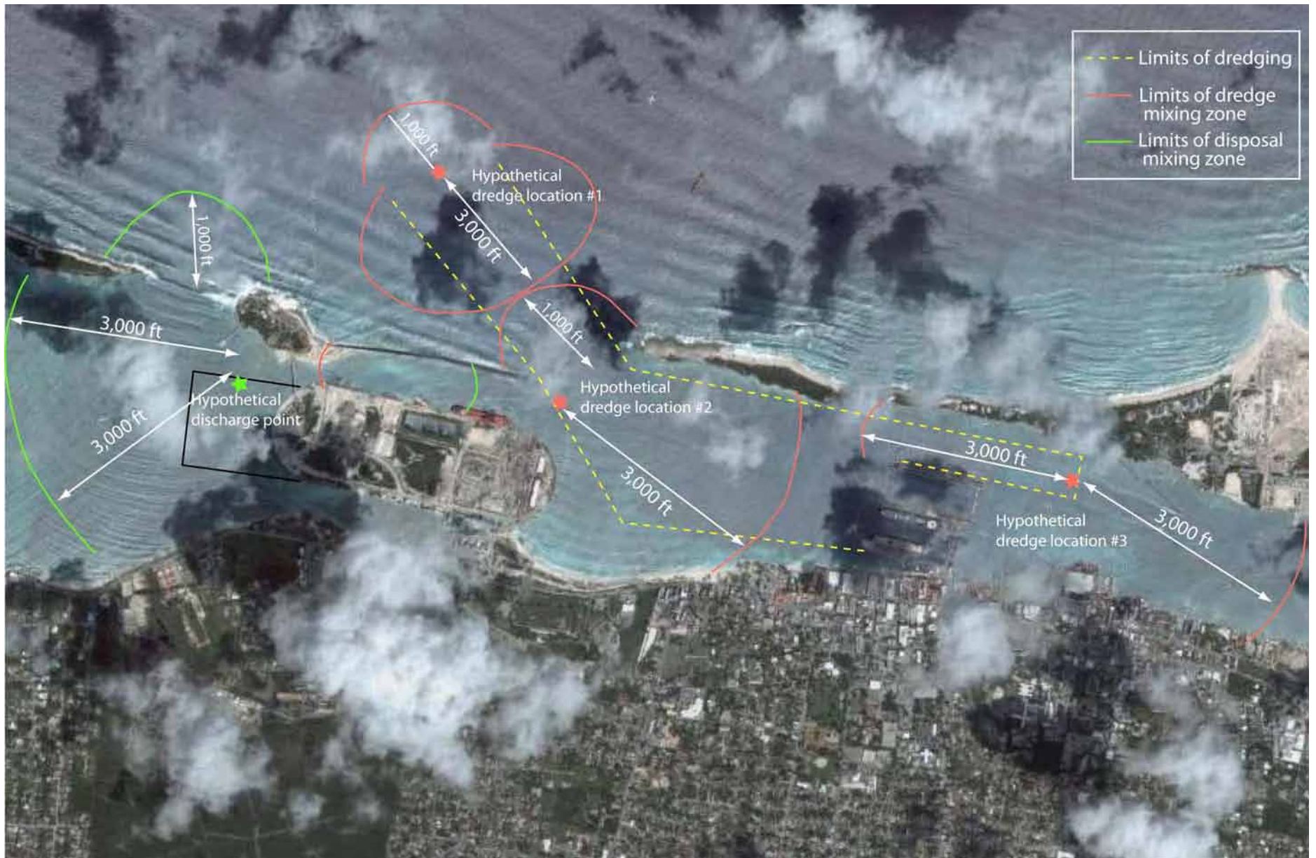
Figure 1. Illustration of disposal and dredge mixing zones. Not to scale. For illustration purposes only.
