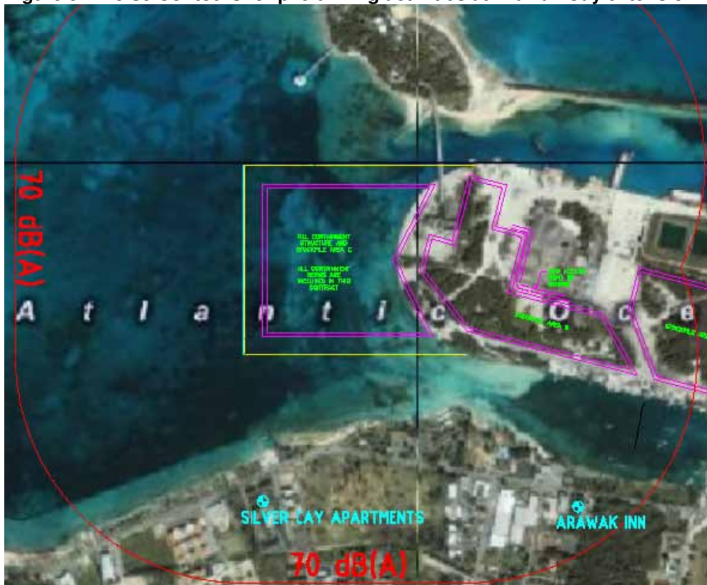
Figure 5.5 Indicating properties most affected by noise from pile driving activities at Arawak Cay extension
