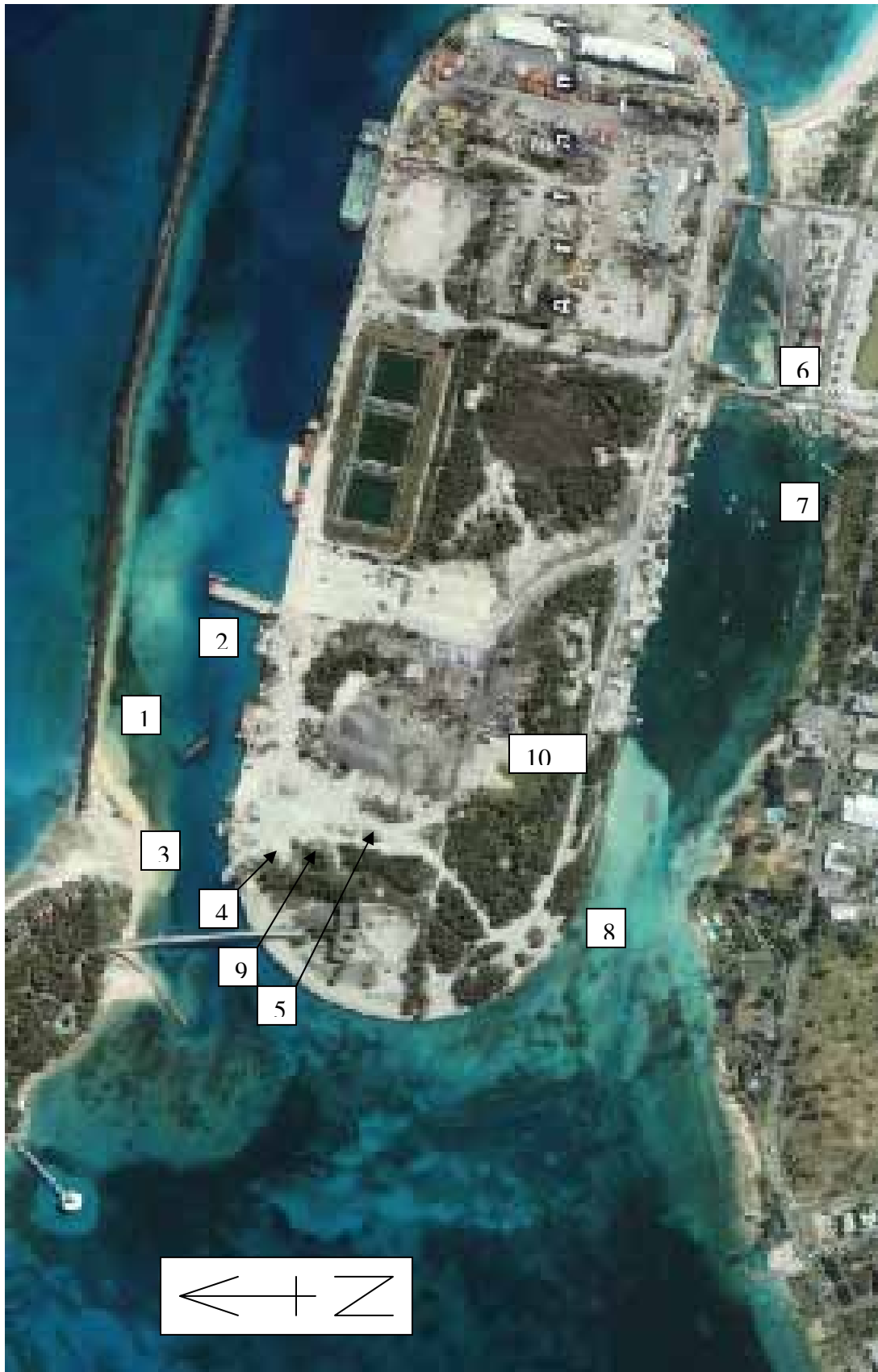
Figure 7.1: Plan of Arawak Cay indicating waste removal locations
